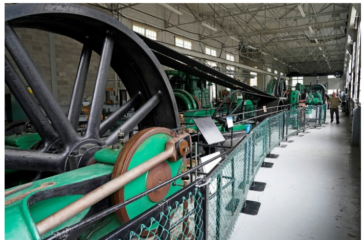
ABOVE: The powerhouse is dominated by a stream-powered pelton wheel driven compressor that delivered fresh air to the underground mine drifts. Connecting the driven end to the compressor is 100-plus-year-old hemp rope.
