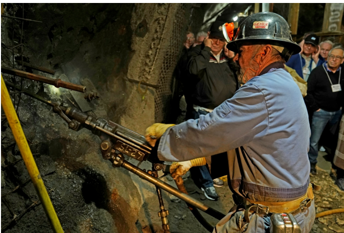
ABOVE LEFT: Bill Roberts operating a pneumatic jackleg drill.
