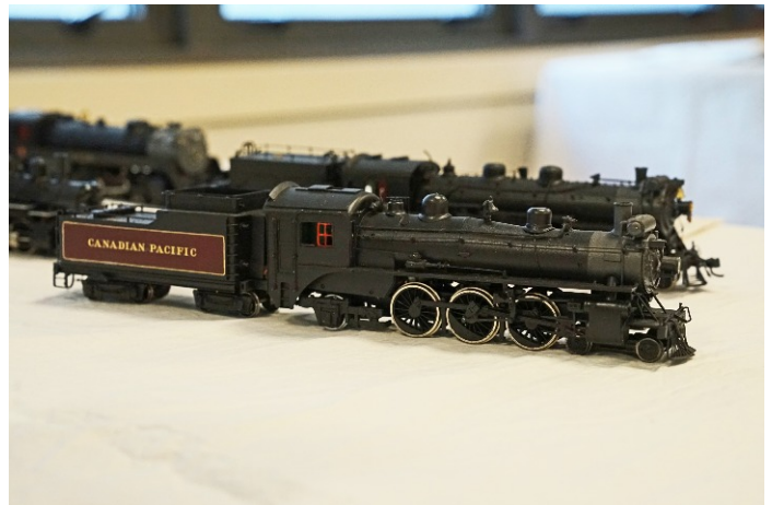
ABOVE: Takahiro Yuasa's CPR 4-6-2 Pacific. Generally, he re-works the frame and motor to create a very smooth drive. On some models, not necessarily this one, he has included ball bearings in the frame for the driver axles. He usually makes the cab doors and roof hatches open and close on working hinges.
