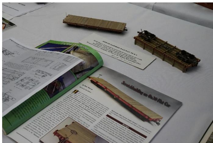
ABOVE: Russ Watson scratchbuilt this On30 flatcar and gondola from home-cut scale lumber, brass wire and commercial detail parts. Scale drawings for a 3 ft gauge Sierra Nevada Wood and Lumber Co. 28 ft flatcar and a 3 ft gauge SP gondola provided the reference dimensions. Russ had his article published in the modelling press.
