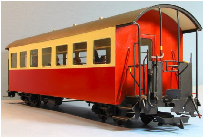
ABOVE LEFT: Brass sides with milled windows and brass wire inserts
