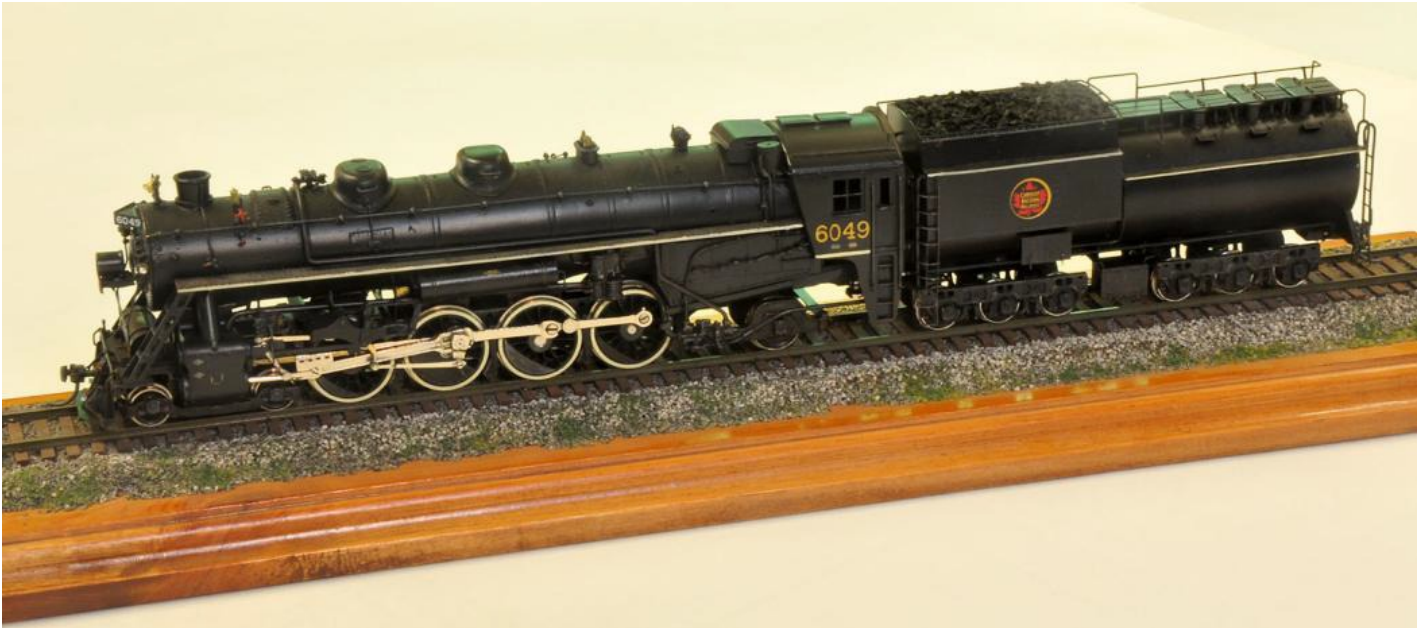
ABOVE: Fireman's side of Kyle Gardiner's model of CNR No. 6049. Note the stoker access door unique to the U-1-e Class below the monogram on the scratch built tender. - Al Lill photos above and below, October 2014
