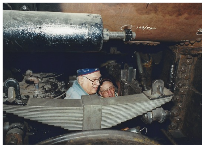
Leaf Spring Inspection
